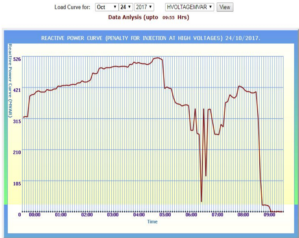
Figure-1: Reactive power injection by Delhi control area to NR grid causing Penalty
